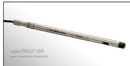
Fig. 3b. An In Situ Aqua Troll 200 data logger. It logged stream height (to estimate hourly stream discharge), temperature and specific conductance of the stream on an hourly interval.
